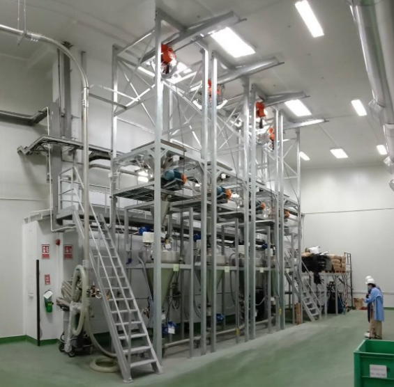
Complete station installed in Bulk Bag Unloading station with Operation & Service platform, Inverter Speed control to be matched with system requirement
